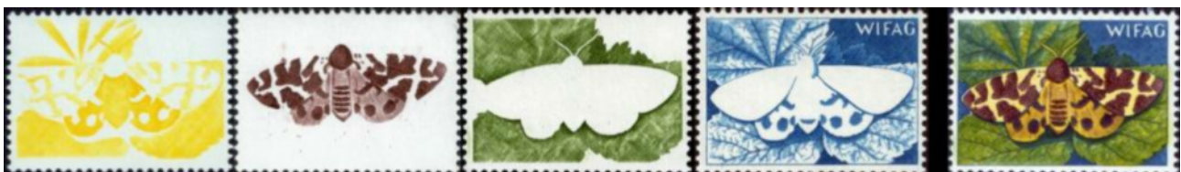
Figure 8: Four WIFAG offset plates required to produce a four-colour print.
