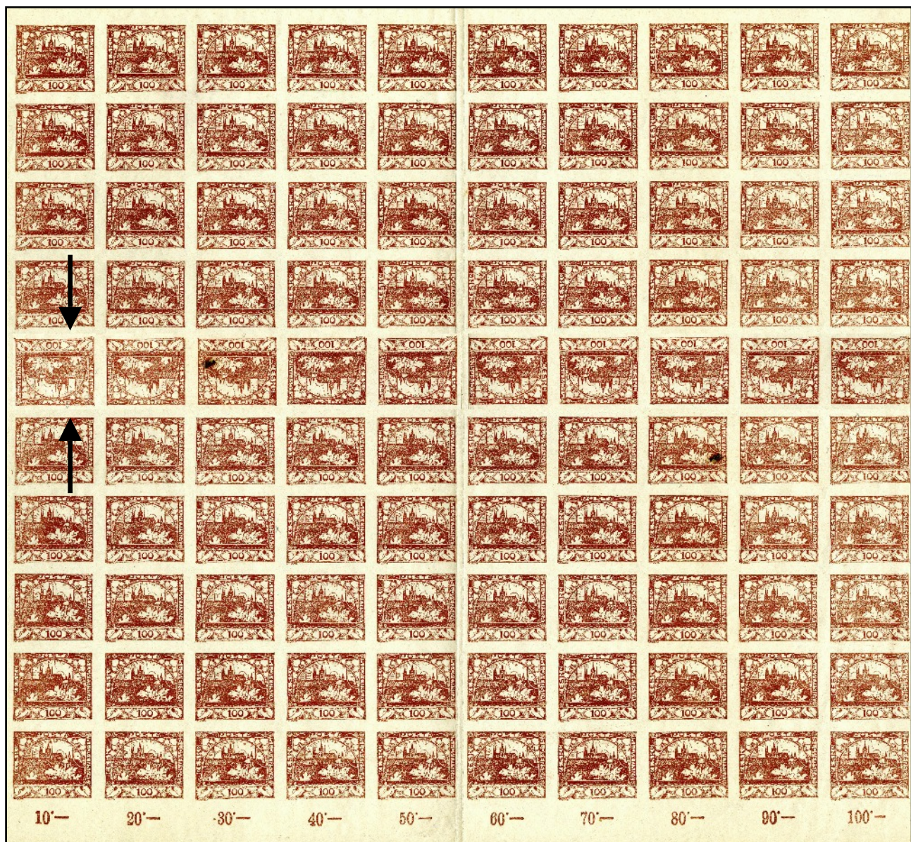
Figure 11: Paper after the second pass. The number of rows inked determined the production of a full or partial pane.
