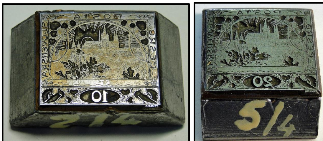
Figure 13: Dies from the 10h card from the Second Regular Issue and the 20h lettercard.
