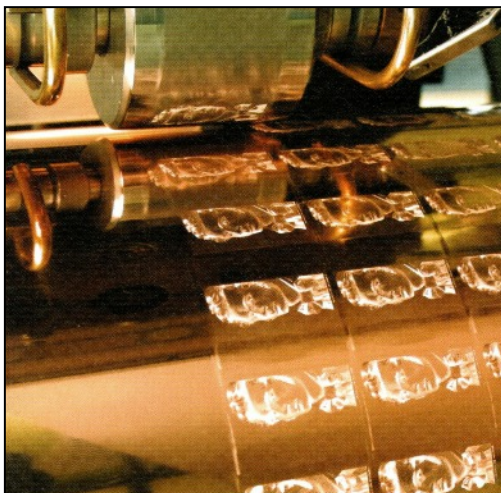
An Embossed Molette Incising Intaglio Clichés. Modern methods do not use positioning marks. Molette images courtesy of Mogens Norbjerg.
